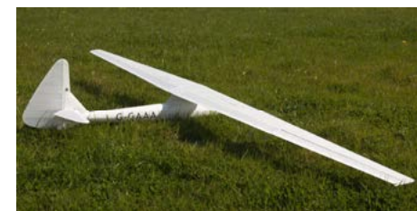
HJORDIS.—High performance sailplane, designed by G. M. Buxton, built by Slingsby Sailplanes in 1935, owned by F. A. Wills and G. M. Buxton. Span, 51 ft.; wing loading, 4 lbs. per sq. ft.
